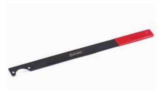
The Schwaben BMW Water Pump Locking Tool many BMW 6-cylinder engines. The tool bolts directly to the water pump pulley using two pump bolts. Its long handle provides added leverage to let you hold the pump stationary while removing the cooling fan nut.
