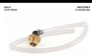
The Schwaben oil filter housing drain tool takes the mess out of oil changes. Thread the drain adapter into the bottom of the filter housing to drain the oil before removing it. The long flexible tube directs drain oil into your catch can to prevent spillage.
